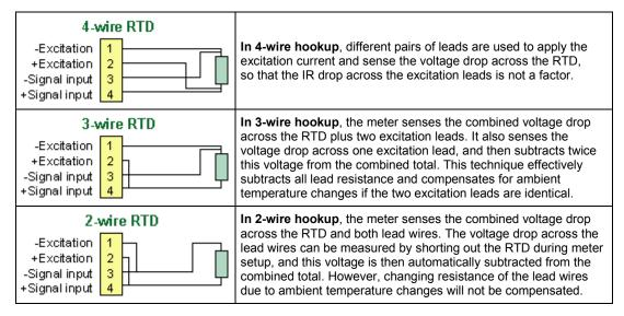
RTD hookup can be via 2, 3 or 4 wires to the J5 connector. The meter applies an excitation current of 256 µA (Pt100 and Ni120) or 5 mA (Cu10).
